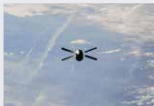
Launch of the 4<sup>th</sup> Automated Transfer Vehicle (ATV), Albert Einstein: Named following a Swiss proposal, it is one of the five ATV spacecraft developed by ESA that have made an essential contribution to the resupply of the ISS. Important ATV components were built by Swiss industry, including the spacecraft structure (RUAG Space), protection against micro meteorites (APCO Technologies), and electronic components (Syderal). © ESA
