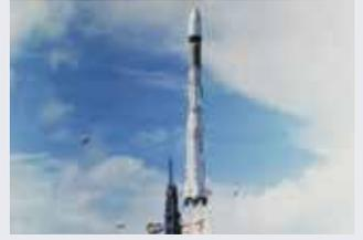
Launcher payload protection – swiss-made: The maiden flight of the European Ariane-1 launch vehicle, featuring a Swiss payload fairing. Ariane-1 was designed primarily to put two satellites into orbit at a time, thus reducing costs. As the size of the satellites grew, Ariane-1 began to give way to the more powerful Ariane launchers. RUAG launcher fairings continue to enjoy success for their reliability to this day. © ESA
