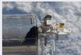
Onboard Columbus: SOVIM, an instrument to observe and study the irradiance of the sun with high precision, stability and accuracy was among the first experiments on board the European Columbus research laboratory attached to the International Space Station ISS. The Swiss instrument was from the Davos Physical Meteorological Observatory. © ESA
