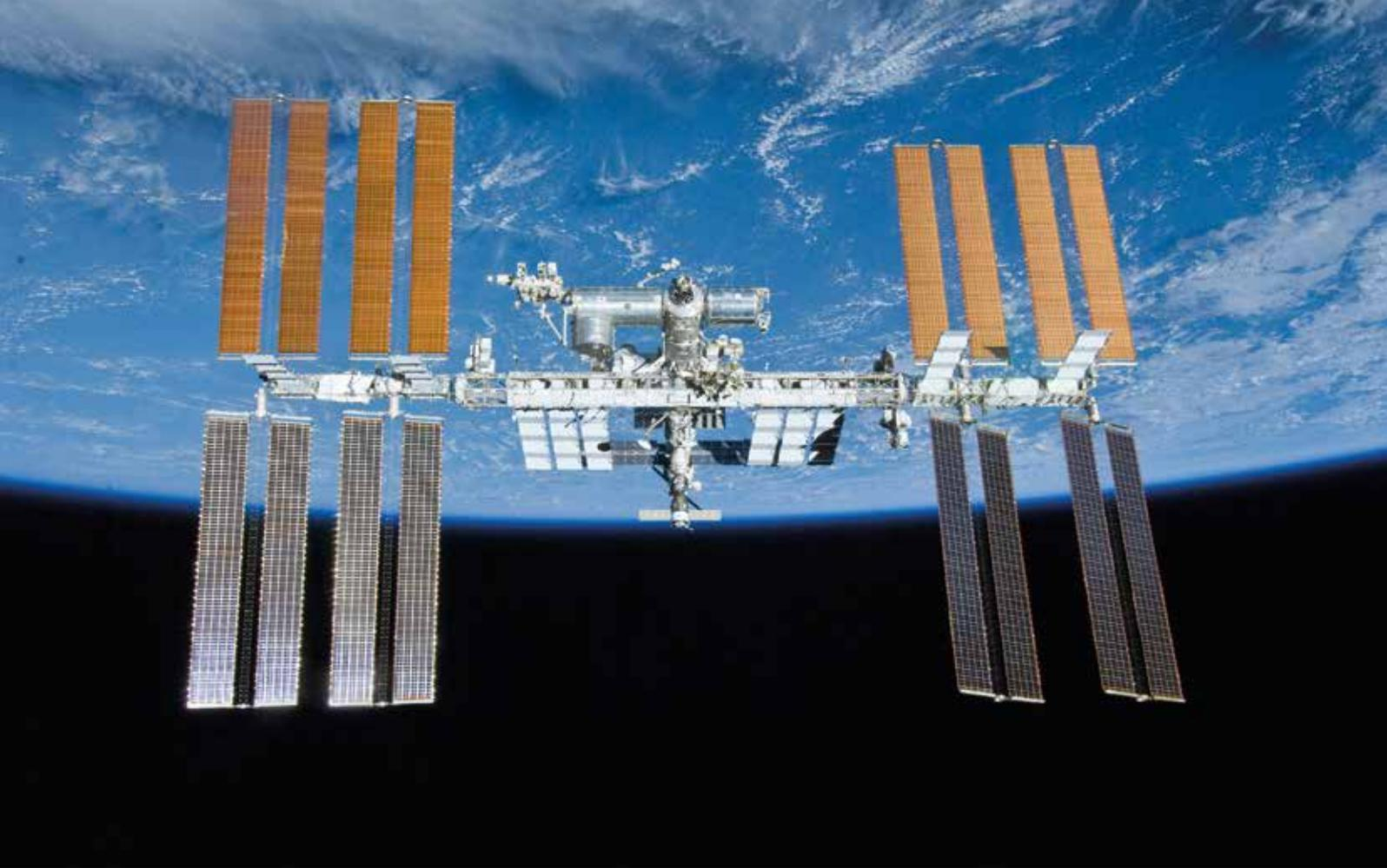
The International Space Station in orbit, photographed from a space shuttle after it undocked in May 2010. The pressurised modules are clearly visible in the middle, and so is the large horizontal truss on which the great wings bearing the solar panels are mounted. A Soyuz spacecraft is visible at one of the zenith port on the station. The European research module Columbus is attached to the starboard side of the station. © NASA
