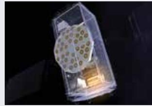
Swiss precision in space: In preparation for deployment of the Galileo System, ESA initiated development of two on-board clock technologies in the 1990s: the Rubidium Atomic Frequency Standard (RAFS) and the Passive Hydrogen Maser (PHM). After the Rubidium clocks had been flown on the first Galileo test satellite launched in 2005, the first PHM clock undergoes in-orbit testing on board the second Galileo test satellite, GIOVE-B. © ESA
