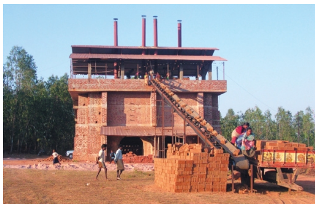
Energy efficient brick technology: Vertical shaft brick kiln
