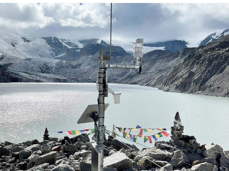
Figure 8: Installation of an early warning system base for glacial lake outburst floods (GLOFs) in Sikkin, India. Photo: SDC/GEOTEST
