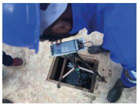
Using the Volaser with the smartphone app in a septic tank in Lusaka, Zambia. © Eawag
